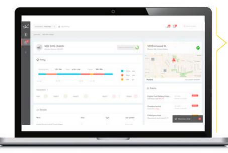
**"UNIT DETAILS"** gives you a status overview of an individual unit. This includes pertinent statistics, as well as fault codes generated during the machine's life cycle, alerts or upcoming maintenance.
