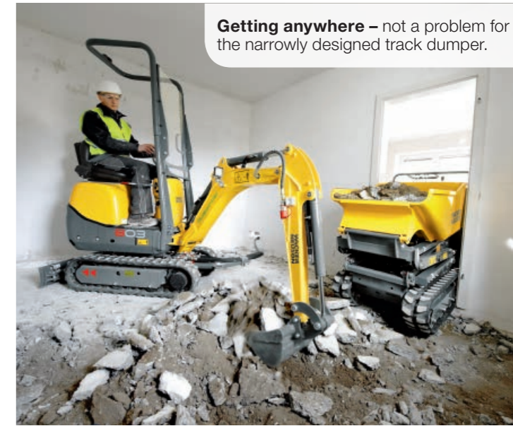
Targeted unloading thanks to the flexible high tip skip – for example in containers.
