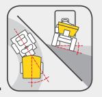
In many applications, rough ground conditions with bumps, small gradients and constricted places is a part of daily operations. For this reason, all wheel dumpers from Wacker Neuson are outfitted with an articulated pendulum joint.
