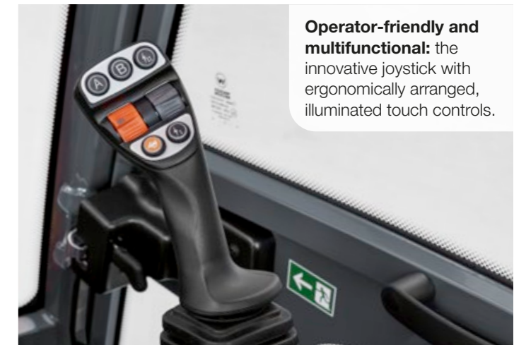
Adjustable joystick console on the operator's seat that swings along.
